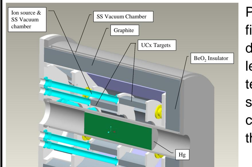
Preliminary design of fission target. Overall dimensions 1m length by 1 m diameter. Length of the spallation source 50 cm, 30 kg of  $^{238}$ UC<sub>x</sub> in the blanket.
